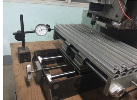
Fig. 11. Y-axis experiment with dial gauge
