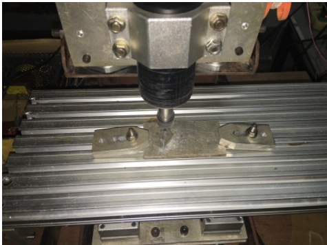
Fig. 14. Cutting sample shape in aluminum
